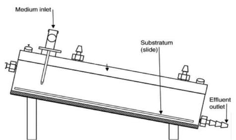
**Figure 6: Close up of Biofilm Reactor Box.** Biofilms grown on the microscope (substratum) slide while the media (with and without donor bacteria drips over the slide through a needle in the medium inlet. Excess media, waste, and unattached bacteria flow out of the biofilm box through the effluent outlet into the waste carboy.
