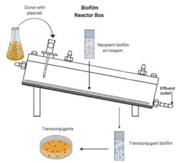
**Figure 3: Drip-Flow Biofilm Mating.** Recipient biofilm grown with a continuous flow of fresh media are exposed to a continuous flow of donor with plasmid for conjugation. Bacterial growth on selective agar results from a successful conjugation.
