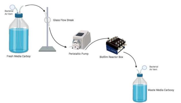
**Figure 5: Drip-Flow Biofilm Reactor Setup.** LB broth flows from the fresh media carboy through the glass flow break, and peristaltic pump through a serious of tubing until it drips into the biofilm reactor box where the recipient biofilm is forming. For conjugation, cultured donor with plasmid is added to the fresh media carboy and follows the same drip procedure. Waste flows from the biofilm reactor box into the waste carboy for sterilization.
