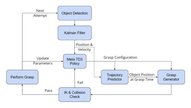
Figure 4.1 - AI Subsystem Flow Diagram
