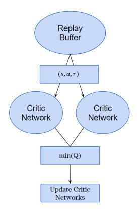
Figure 2.3 - TD3 Critic Update Diagram
