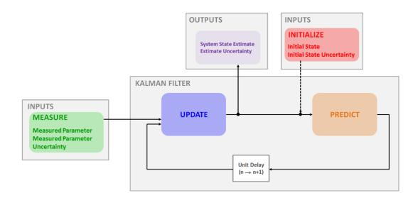
Figure 4.3 - Kalman Filter Block Diagram
